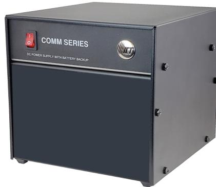
The ICT Backup Series combines backup batteries, power supply, and enclosure, all pre-assembled into an integrated compact solution. The power supply provides DC power to the radio while charging the internal battery, then if AC fails it will automatically and seamlessly transfer the load to the battery for up to 8 hours (depending on radio model and current draw).
